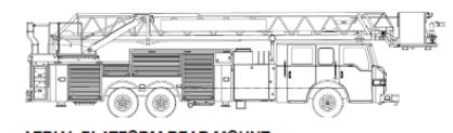
AERIAL PLATFORM REAR MOUNT GVW: 33.7 T (min), 43 T (max) Length: 46' (min), 48' (max)
